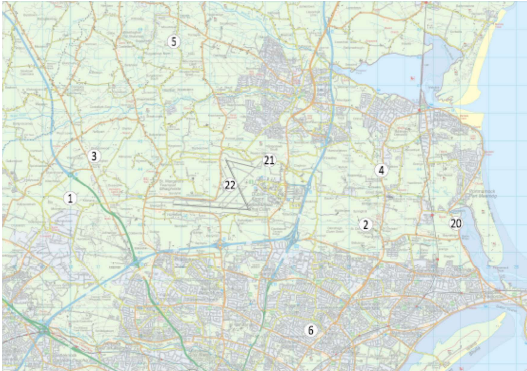
Figure 13-2: Permanent Noise Monitoring Terminals at Dublin Airport (2018)
