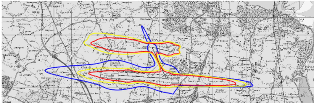
Figure 13-6: 65 dB L_{den} Noise Contours, 2018 (blue), 2025 Permitted (yellow) and 2035 Permitted (red)
