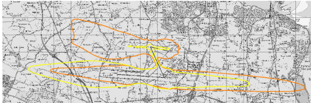
Figure 13-10: 55 dB L_{night} Noise Contours, 2025 Proposed (orange) and 2025 Permitted (yellow).
